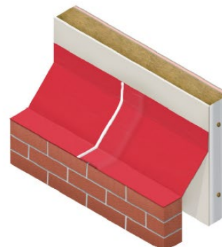
5. Install adjacent Visqueen Zedex Non-Combustible DPC cavity tray and seal lap
