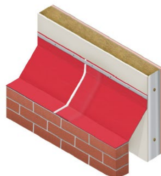
6. Install Visqueen Non-Combustible Fixing Strip and bed DPC in mortar
