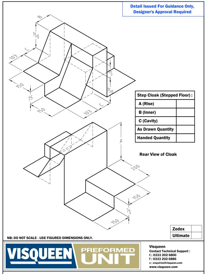
Project: Standard Detail: Suspended Slab - Typical Gas Protection Detail - Preformed Step Cloak.
