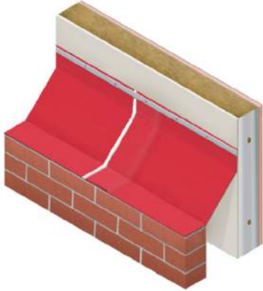
Diagram 5 - lap joint, including Visqueen Non-Combustible Fixing Strips
